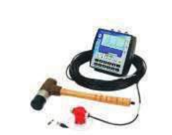
Pile Integrity Test
