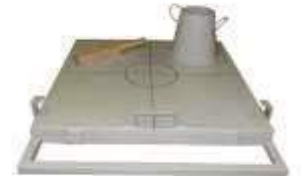
Concrete Flow Table Test Set
